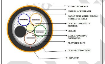
3.9.4 Strength Member: Solid FRP non - metallic strength member shall be used in the center of the cable core. The strength member in the cable shall be for strength and flexibility of the cable and shall have anti buckling properties. The FRP shall keep the fibre strain within permissible values. The strength member(FRP) shall be as per the Standard No. TEC 89010:2021(or latest release) and the subsequent amendments, if any. The size of FRP shall be as per Annexure – I.
